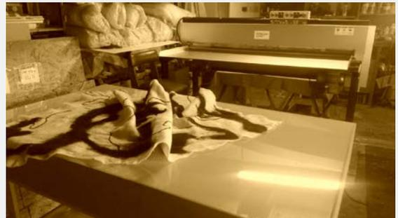
The FeltLOOM Pro-Line 66 has a 66" bed and 800 needles, enabling varying sizes of products to be created as well as varying thicknesses (Max ½ in thick).
