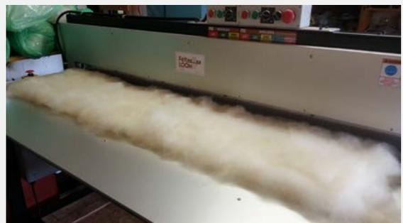
The process of felting on our Feltloom requires a premade batt (*which can be made by either Quenti Mill or Serena Alpacas - the size will depend on the size of the drum at each mill*). Generally the batts are approximately 1mx60cm. Batts can be joined together for a longer and/or wider piece of fabric should this be needed.
